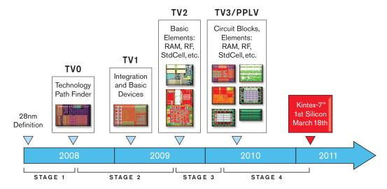
Xilinx's unique PPLV approach contributed to the optimization of process parameters while also providing better circuit-modeling enhancement for the 7 series designs. To further understand the challenges of the 28nm generation, test chips also enabled learning cycles relating to:
