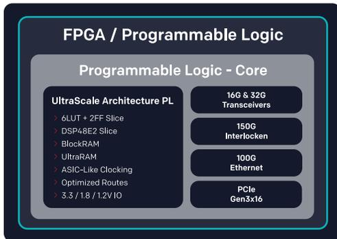
**XQ UltraScale Architecture FPGAs (Programmable Logic)**
