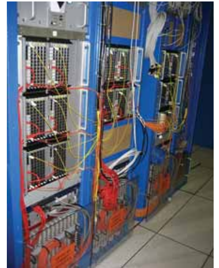
Figure 4 – One of many racks containing the TMU cards that filter and track trajectory data from the lead ion collision.
