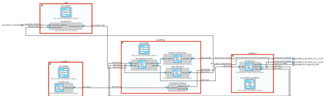
VSI generated runtime & data transport hardware, work in unison to transport the data between blocks executing in CPU and FPGA and between FPGA and FPGA.
