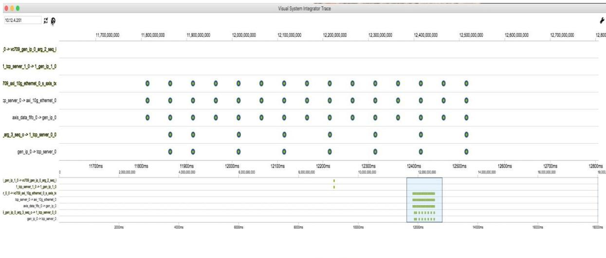
Use VSI's integrated system level *"trace"* application shows events across the entire system , both hardware and software , on a single timeline. With this capability the developer can quickly identify functional problems or performance bottle necks.
