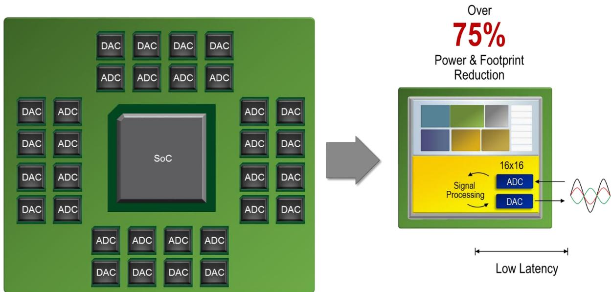
ADC and DAC integration, coupled with integrated digital signal processing engines on 16nm FinFET+ address the low latency requirements for rapid response in A2AD (Anti-Access and Area Denial) events. High channel count systems can achieve over 75% reduction in power and footprint. The single chip, modular 16x16 T/R module can then be arrayed into a 2D array for a fully programmable digital radar platform.
