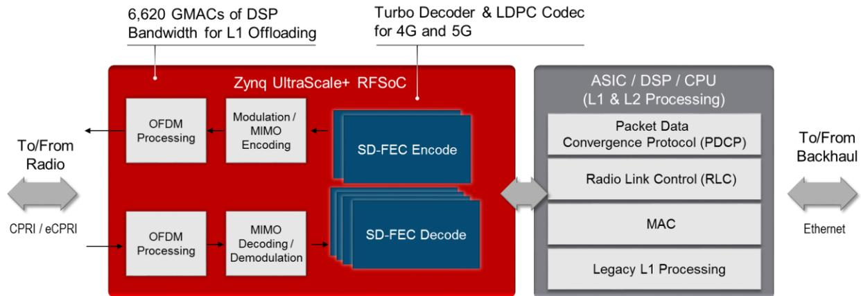
Power efficiency is critical in baseband processing, and a single Zynq UltraScale+ SD-FEC core in an LDPC configuration would take 300K logic cells in programmable logic while consuming 5X the dynamic power. RFSocS realize 10-20X throughput vs. soft cores while meeting the stringent power and thermal constraints for centralized baseband.
