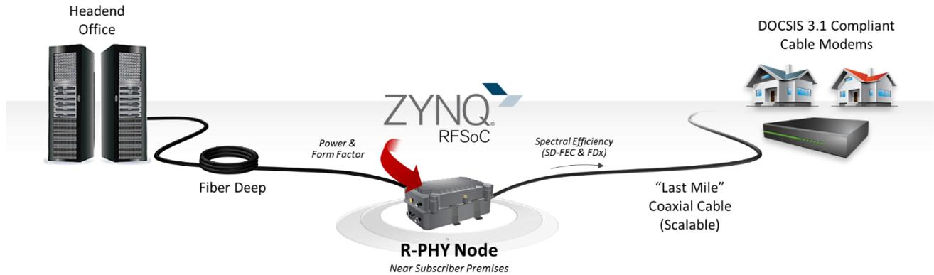
As a multi-channel system of varied configurations, R-PHY demands power efficiency given the greater number of nodes vs. headend equipment. A basic 1 downstream x 2 upstream channel system with Zynq UltraScale+ RFSOC can reduce power and footprint of the Remote-PHY Device by 30-50% vs. a traditional FPGA/ASSP implementation through integration of data converters, all while offering scalability of channel count for flexible provisioning of varied services and number of subscribers.
