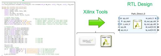
> **Tools:** SDSoC and Vivado HLS enabled motor control algorithm written in C/C++ code to be made into hardware implementation
