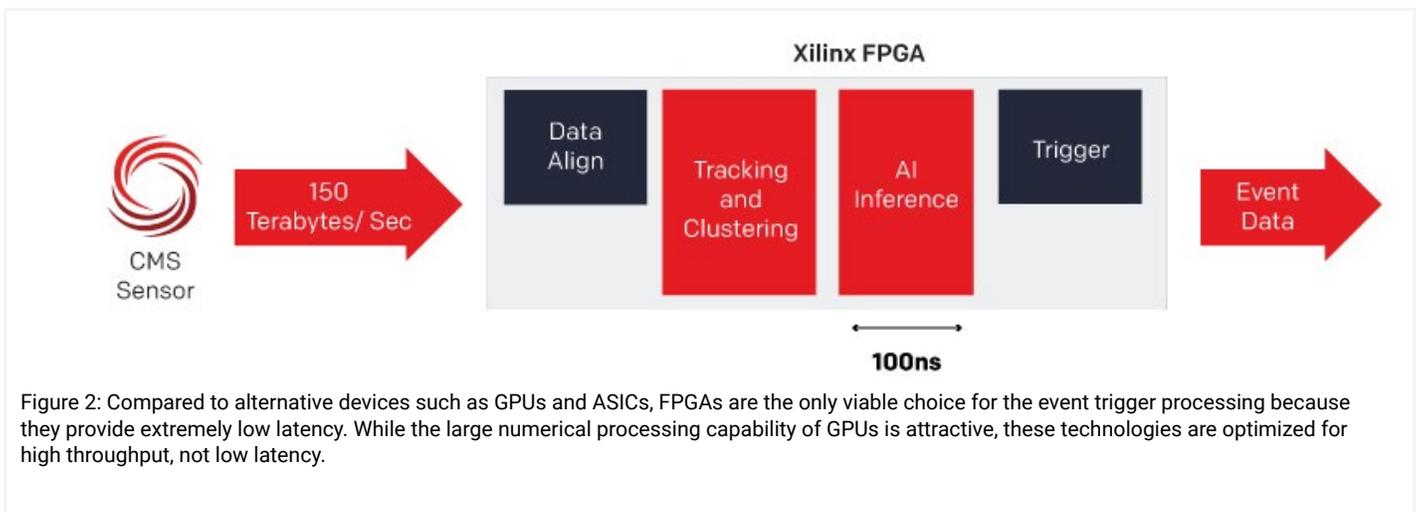
Figure 2: Compared to alternative devices such as GPUs and ASICs, FPGAs are the only viable choice for the event trigger processing because they provide extremely low latency. While the large numerical processing capability of GPUs is attractive, these technologies are optimized for high throughput, not low latency.
