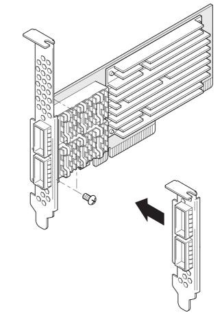
An optional 1PPS bracket and cable assembly, Solarflare part number SOLR-PPS-DP40G, is available for Solarflare dual-port QSFP+ server adapters. For detailed fitting instructions, refer to the *Solarflare Server Adapter User Guide*.
