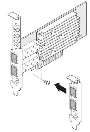
An optional 1PPS bracket and cable assembly, Solarflare part number SOLR-PPS-DP10G, is available for Solarflare dual-port SFP28 server adapters. For detailed fitting instructions, refer to the *Solarflare Server Adapter User Guide*.
