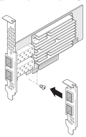
An optional 1PPS bracket and cable assembly, Solarflare part number SOLR-PPS-DP10G, is available for Solarflare dual-port SFP28 server adapters. For detailed fitting instructions, refer to the *Solarflare Server Adapter User Guide*.
