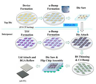
Figure 3. Simplified Package Assembly Process Flow
