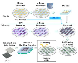
Figure 9. Process Flow with Additional C4 Probe Test Point
