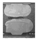
Figure 6. Example of uBump Open Caused by Contamination
