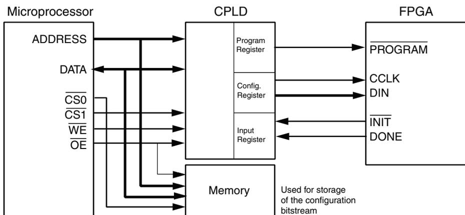
Figure 9: Slave Serial Configuration
