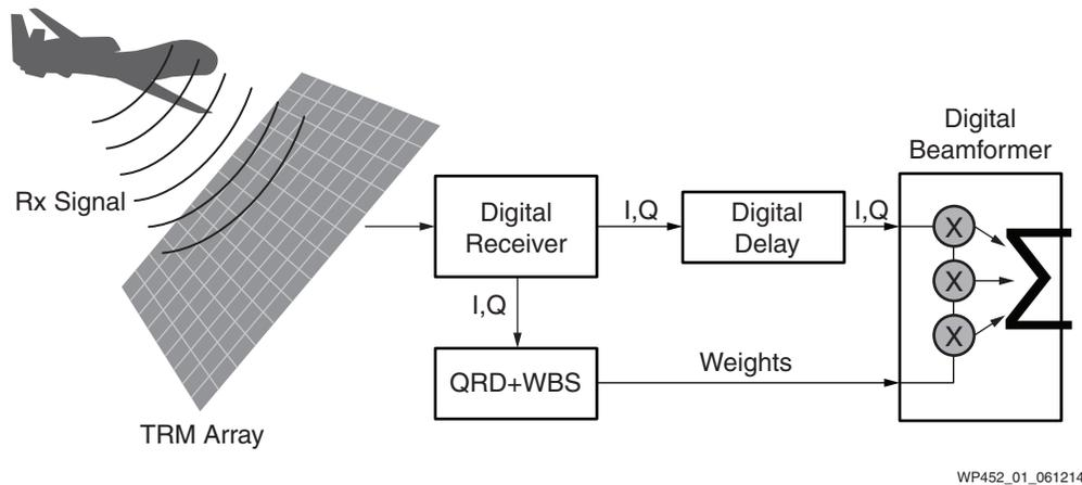
Figure 1: High-Level Overview of Adaptive Digital Beamforming
