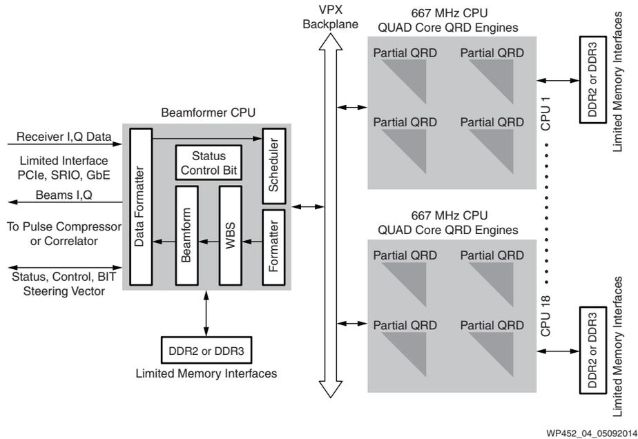
Figure 4: Adaptive Beamformer Architecture Using 18 CPUs (72 Cores)
