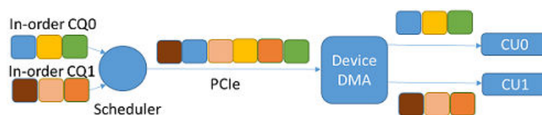
Figure 39: Example with Two In-Order Command Queues
