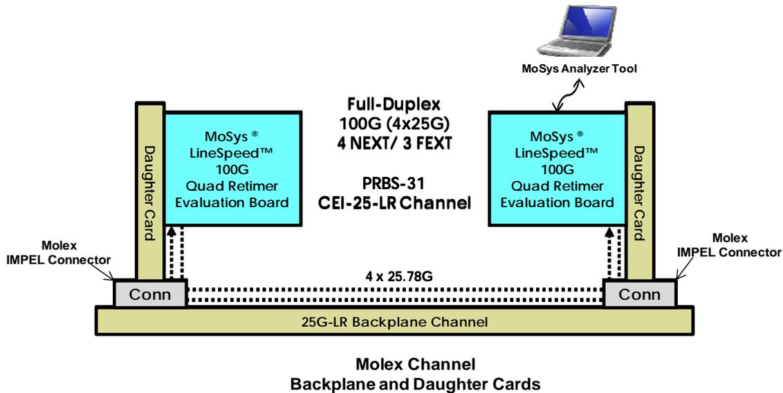
**Figure 17: Demo 8 Block Diagram**
