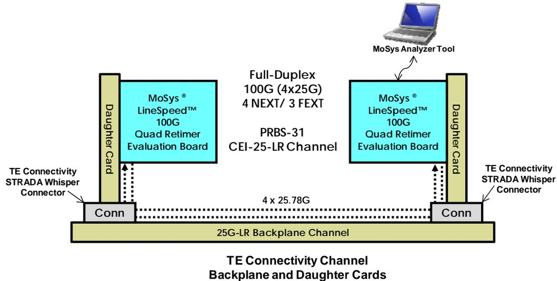
**Figure 18: Demo 9 Block Diagram**
