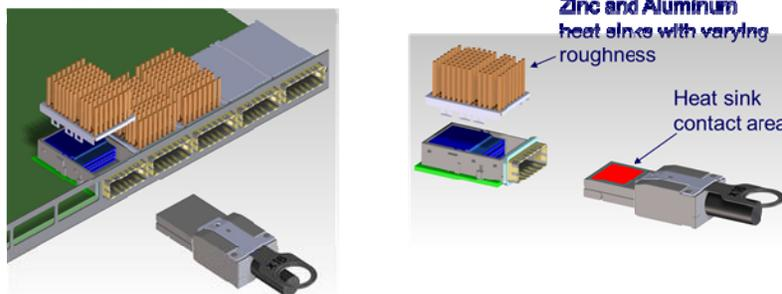
Figure 15: Demo 6 - Thermal Pluggable Module
