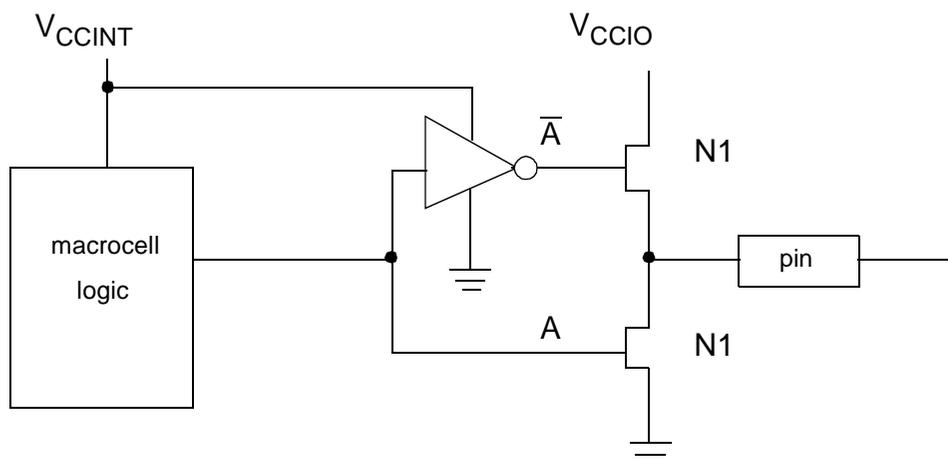
**Figure 4: Close-up of Simplified N-Channel Output Stage (Diodes not shown)**
