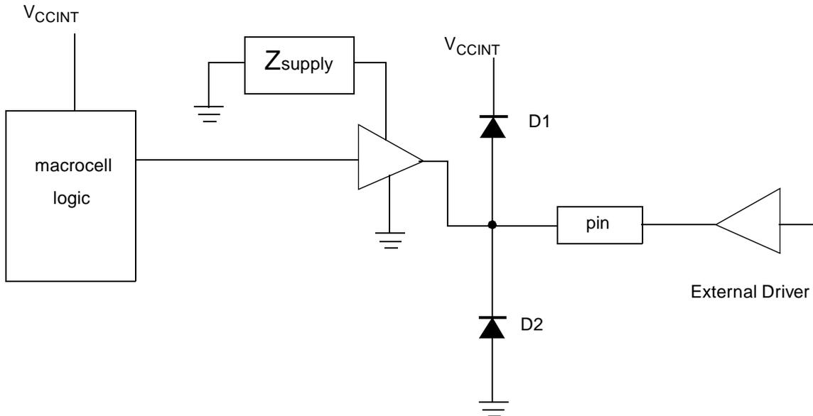
Figure 2: XC9500 Output Driver with  $V_{CCIO}$  turned off (Input Receiver not shown)
