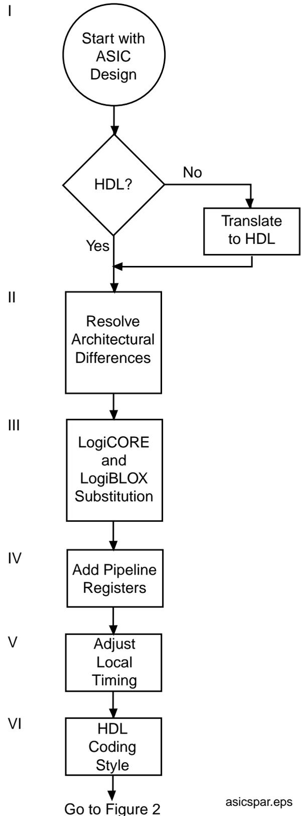
Figure 1: ASIC-to-Spartan Adaptation Flow
