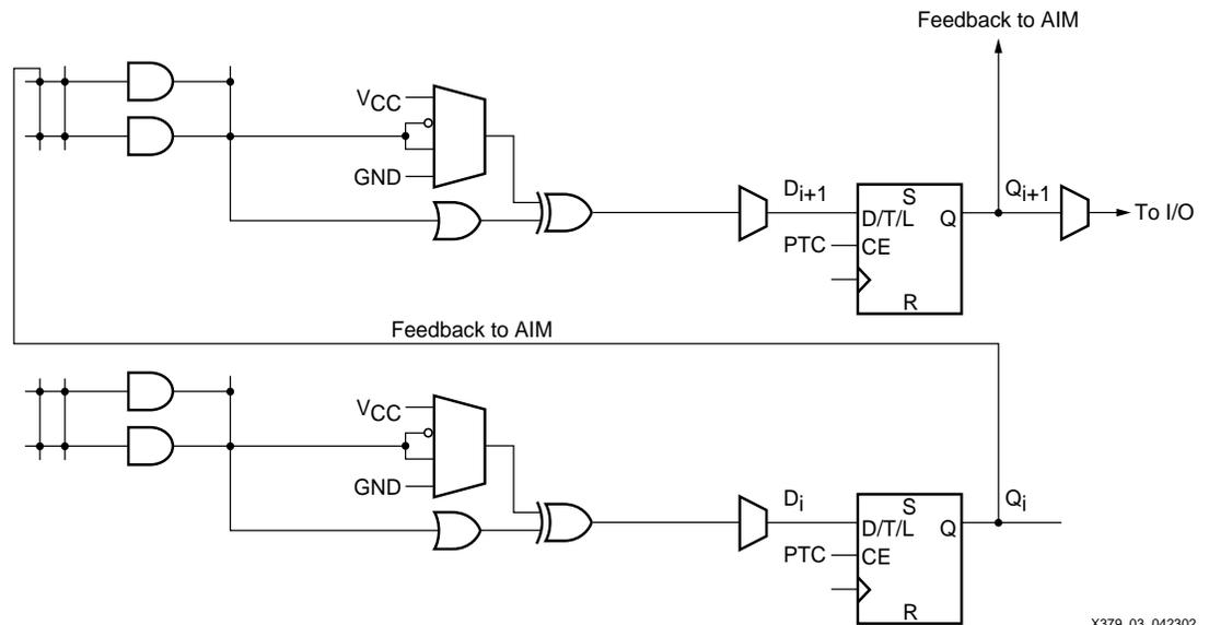
Figure 5: Simple Shift Register
