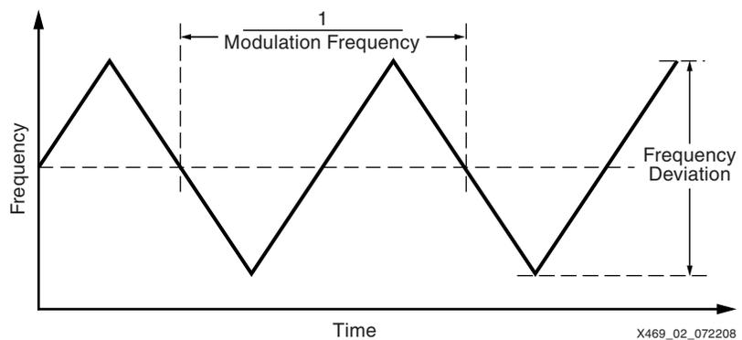
Figure 2: Spread-Spectrum Triangular Modulation Profile
