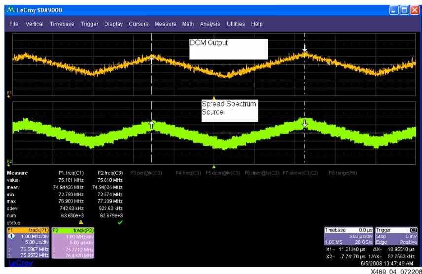
Figure 4: Tracking DCM Frequency Over Time
