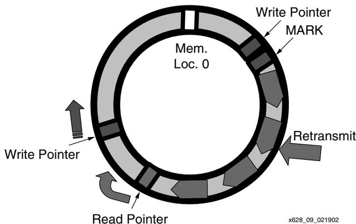
**Figure 9: MARK and Retransmit Operation**
