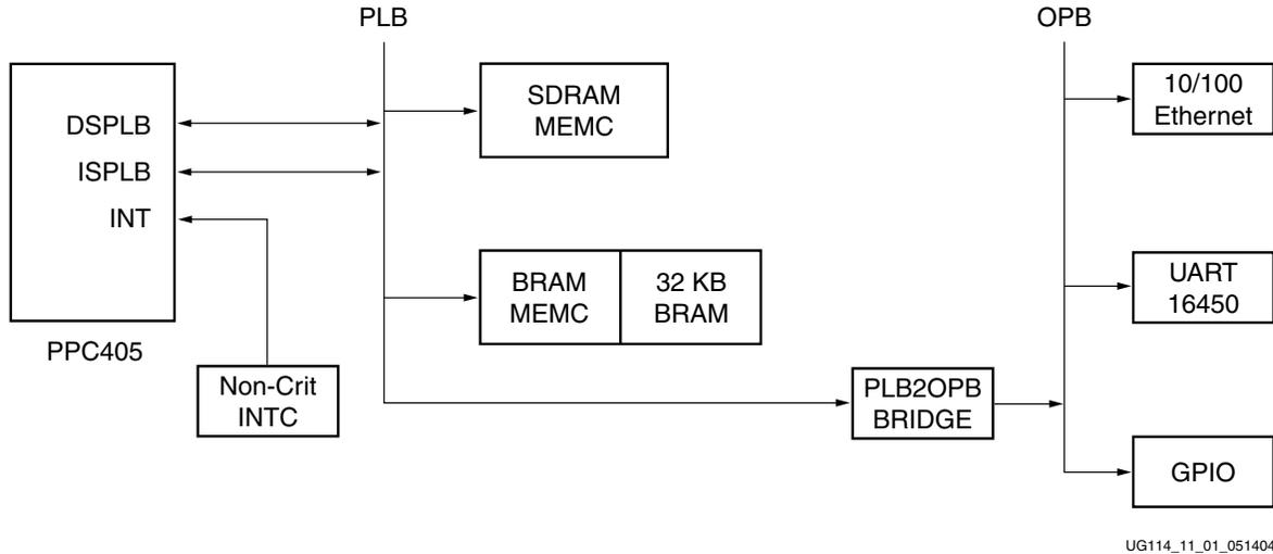
Figure 2: PowerPC System Design for lwIP-Based ECHO Server
