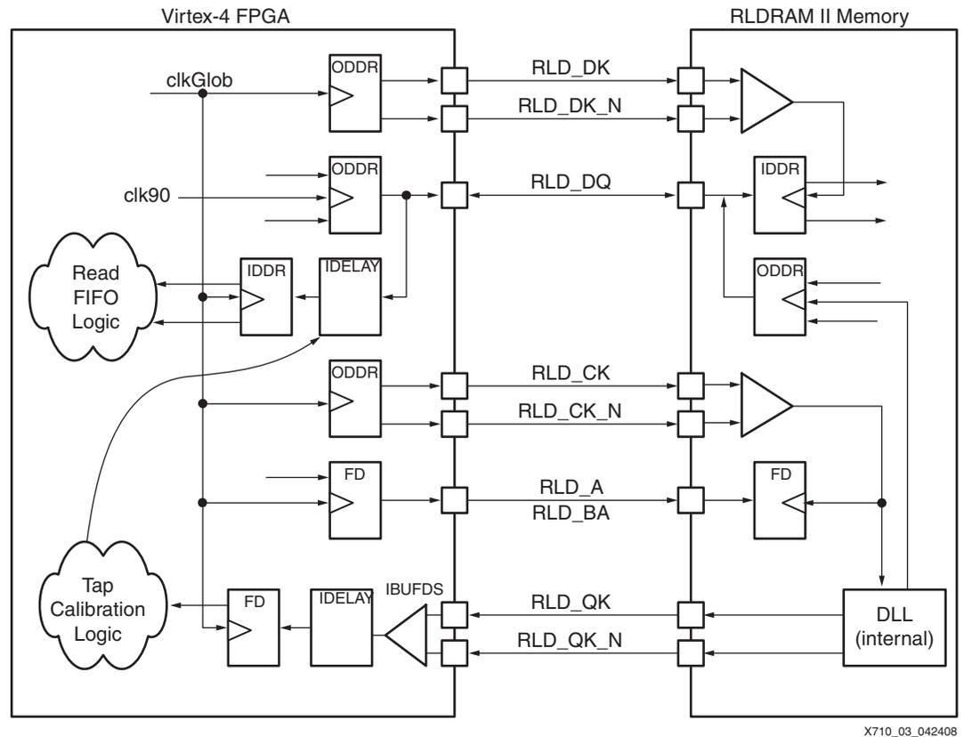
Figure 5: Virtex-4 FPGA and Memory Timing Model
