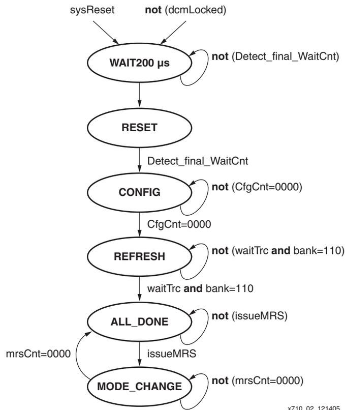
**Figure 3: State Diagram for the Reset/Init Machine**
