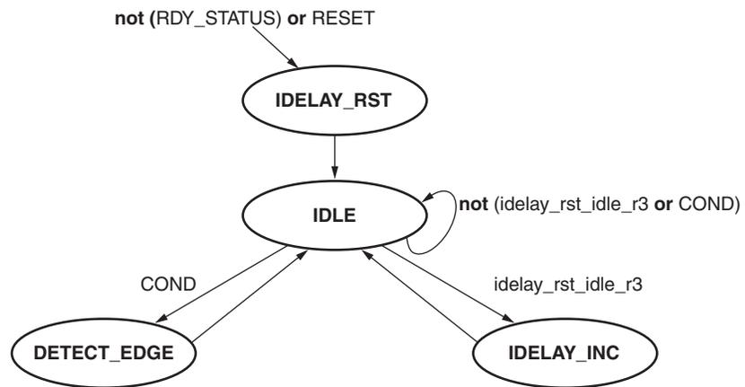
**COND** = idelay\_inc\_idle\_r3 or (detect\_edge\_idle\_r3 and not (second\_edge\_r1) and not (tap\_counter = 111111))
