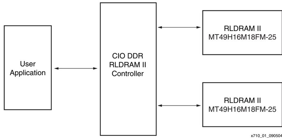
Figure 1: CIO DDR RLDRAM II Controller (Top Level)
