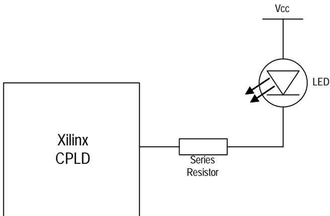
Figure 2: Xilinx CPLD Driving an LED
