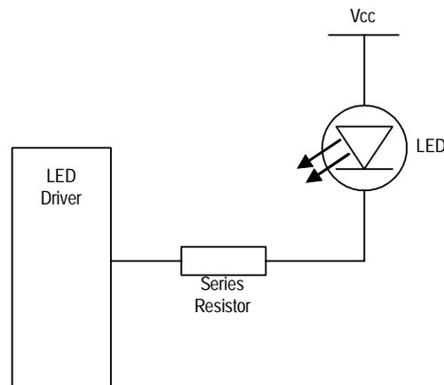
Figure 1: Traditional LED Driver Setup
