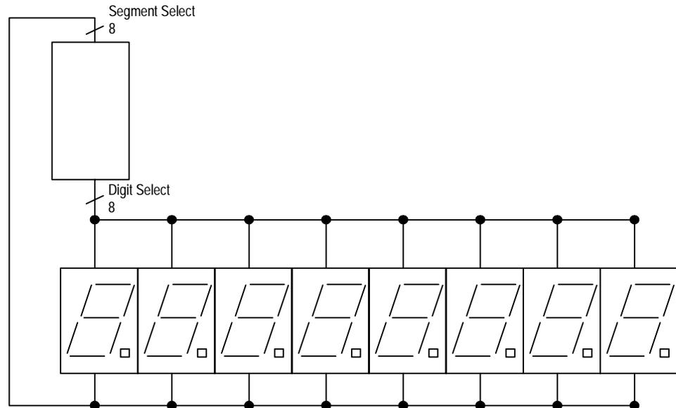
Figure 4: 8-digit 7-segment Display Driver with Data Interface
