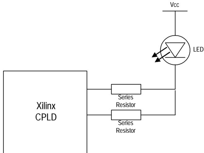
Figure 3: Ganged Multiple Outputs Together for Greater Drive Strength
