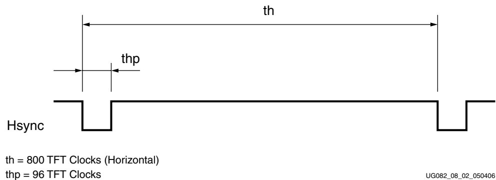
Figure 8-2: Hsync and TFT Clock
