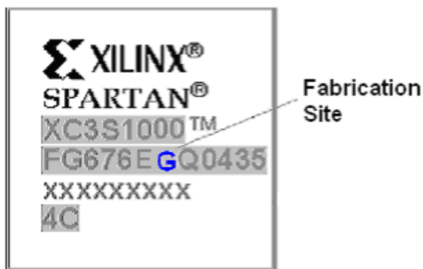
Marking Diagram for 300 mm Wafer Fabrication Facility
