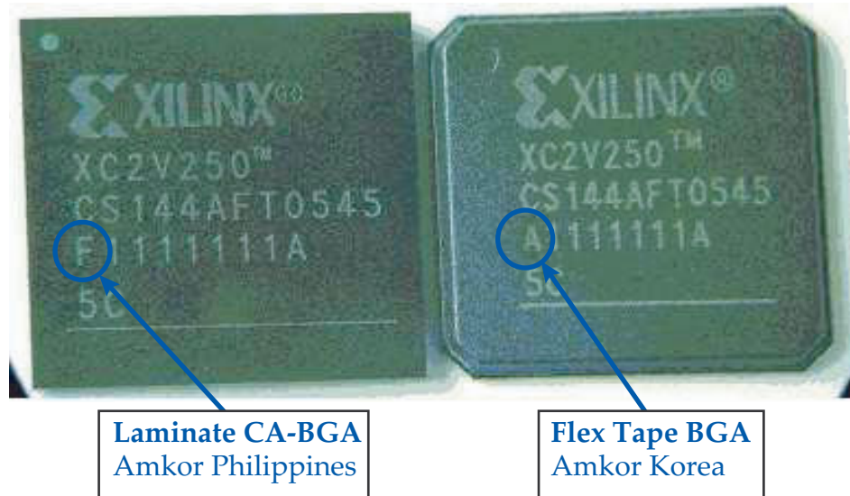
Figure 1: Package Top Mark Showing Assembly Site Code
