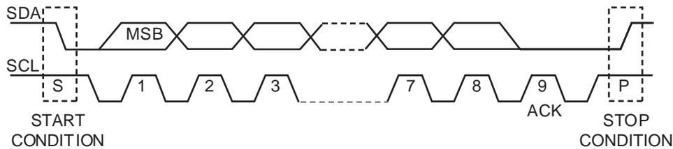
Figure 2: Data Transfer on the IIC Bus
