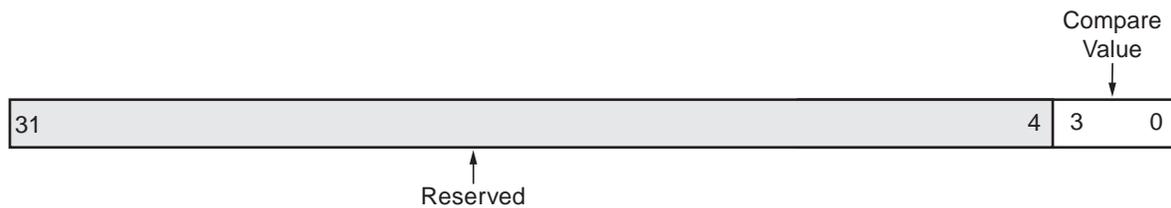
Figure 14: Receive FIFO Programmable Depth Interrupt Register (RX\_FIFO\_PIRQ)
