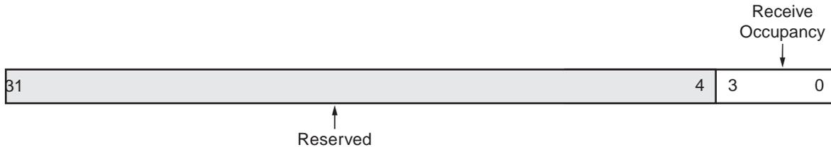
Figure 13: Receive FIFO Occupancy Register (RX\_FIFO\_OCY)
