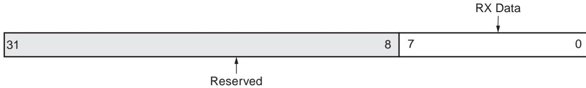
Figure 9: Receive FIFO (RX\_FIFO)
