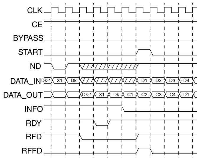
Figure 7: Handshaking Signal Timing
