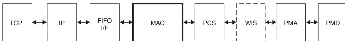
Figure 1: Typical Ethernet System Architecture
