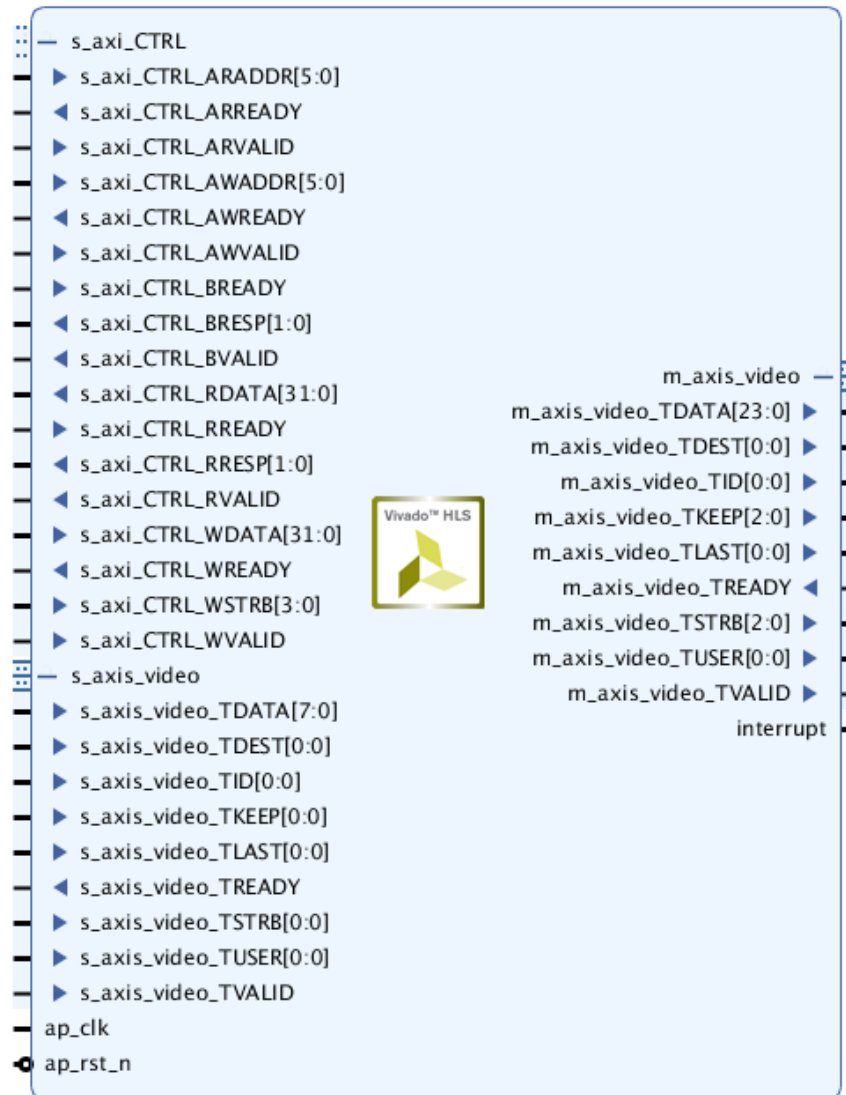
Figure 2-1: Sensor Demosaic Core Top-Level Signaling Interface
