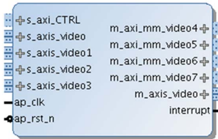
Figure 2-1: Video Mixer I/O Diagram
