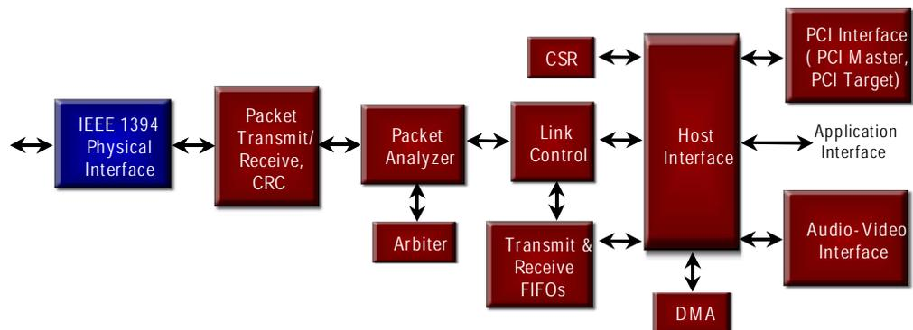
Figure 3: IEEE 1394 Link Controller and Physical Layer Interface
