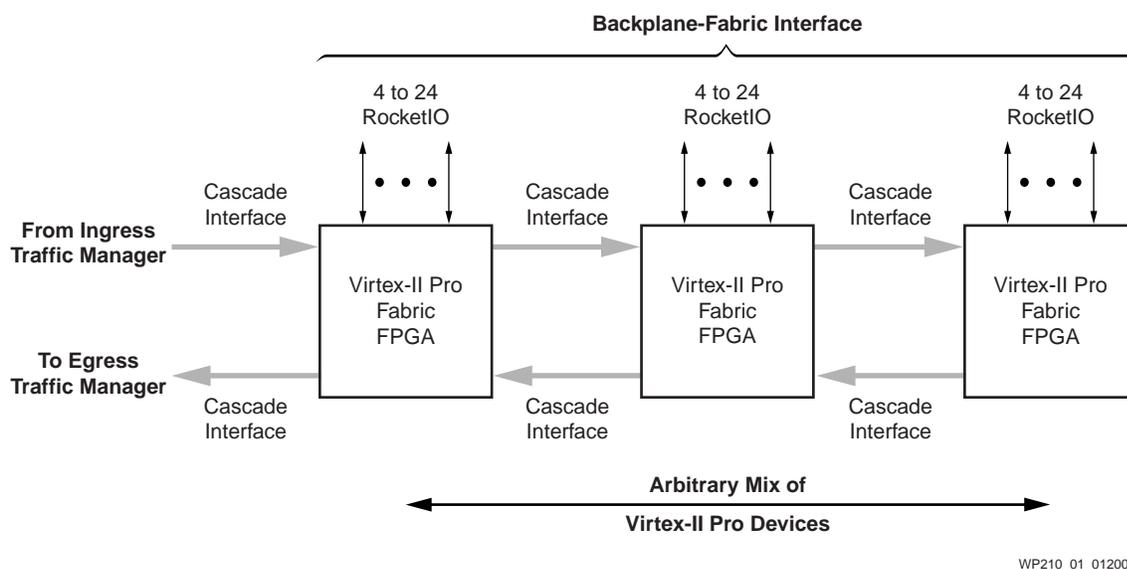
**Figure 1: The mesh fabric reference design can be implemented in a single FPGA or multiple, daisy-chained FPGAs allowing scalability**
