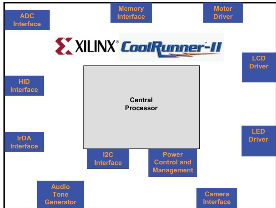
Figure 2: Functions Performed by a CoolRunner-II CPLD
