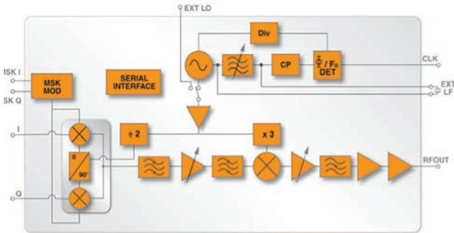
Figure 3 – HMC6300 60-GHz transmitter IC block diagram
