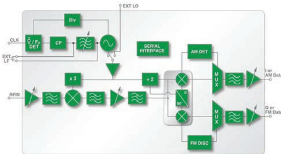
Figure 4 – HMC6301 60-GHz receiver IC block diagram
