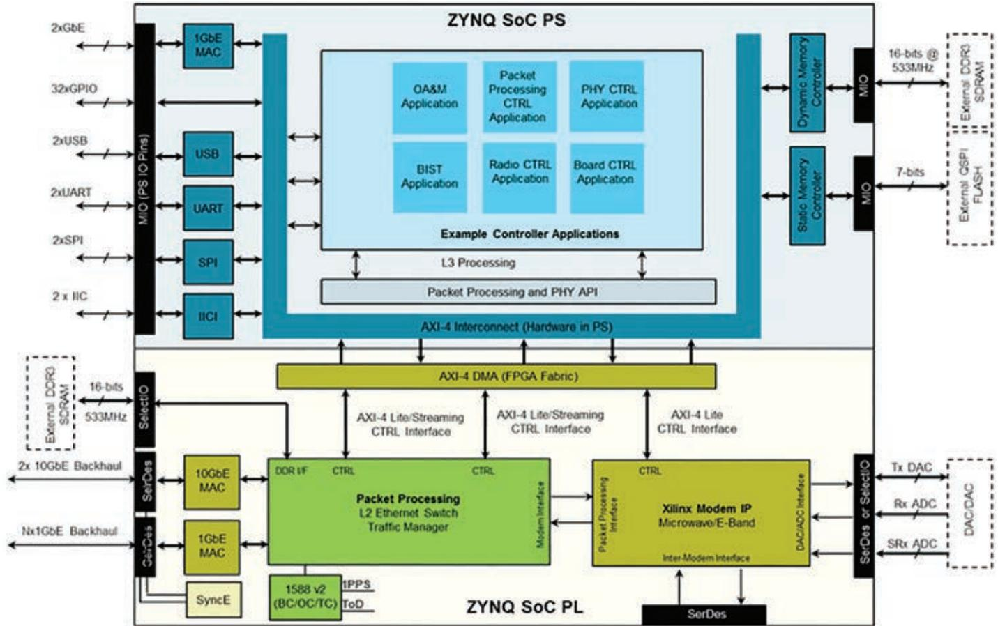
Figure 2 – All Programmable SoC for wireless modem applications
