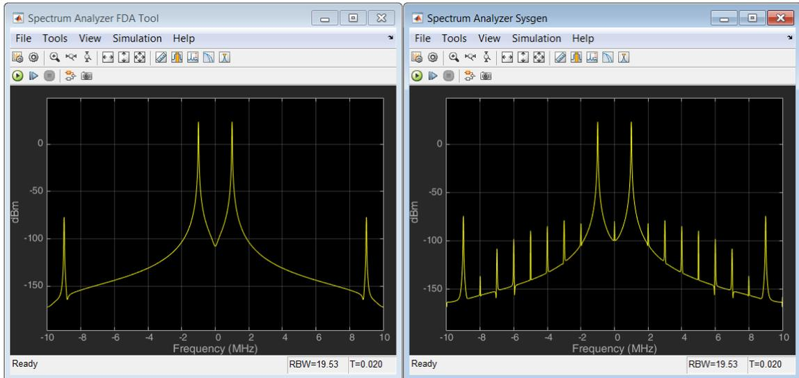
The results are shown above, on the right hand side (in the Spectrum Analyzer SysGen window), and differ slightly from the original design (shown on the left in the Spectrum Analyzer FDA Tool window). This is due to the quantization and sampling effect inherent when a continuous time system is described in discrete time hardware.
