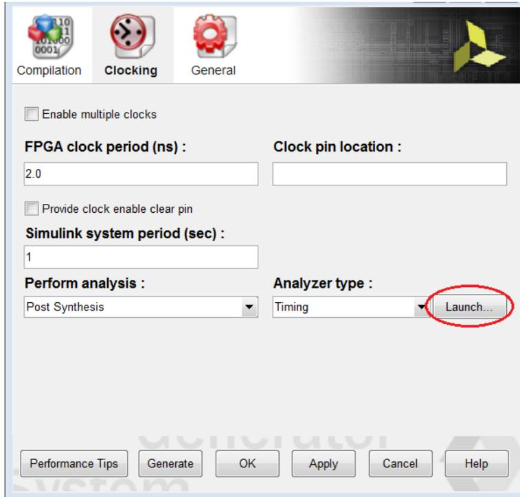
**Note:** If you relaunch the Timing Analyzer window, make sure that the Analyzer type field is set to Timing. The table that opens will display the results stored Target directory specified in the System Generator token dialog box, regardless of the option selected for Perform analysis (Post Synthesis or Post Implementation).
