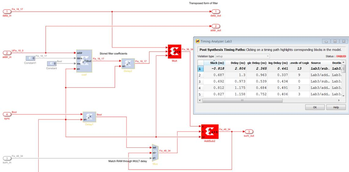
13. Double-click the second path in the Timing Analyzer table and cross-probe, the corresponding highlighted path in green which indicates no timing violation.
