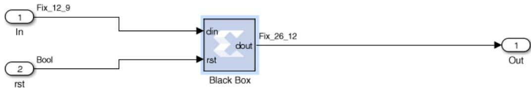
20. From the Black Box block parameter dialog box, change the Simulation mode field from **Inactive** to **Vivado Simulator** and then click **OK**.
