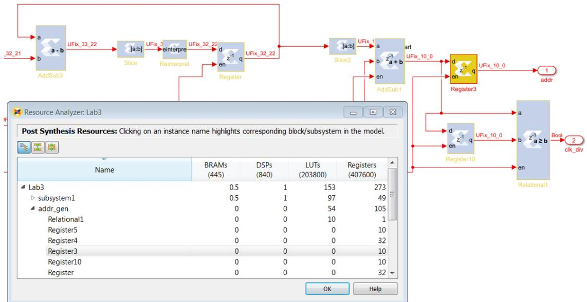
★ **IMPORTANT!** If the Resource Analyzer window or the Timing Analyzer window opens and no information is displayed in the window (table cells are empty), double-click the System Generator token and set the Target directory to a new directory, that is, a directory that has not been used before. Then run the analysis again.
