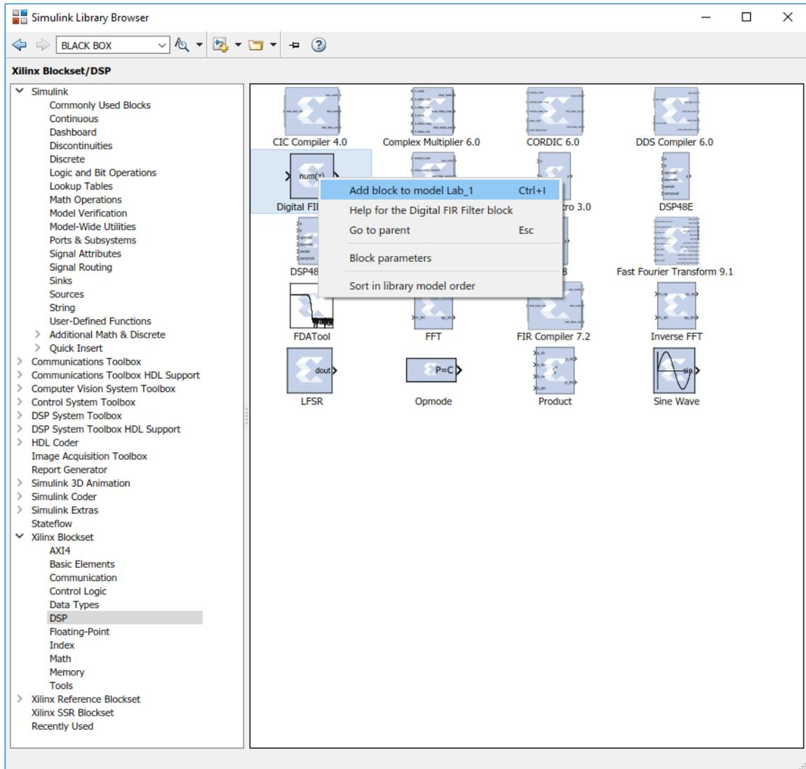
You can define the filter coefficients for the Digital FIR Filter block by accessing the block attributes—double-click the **Digital FIR Filter** block to view these—or, as in this case, they can be defined using the **FDATool**.
