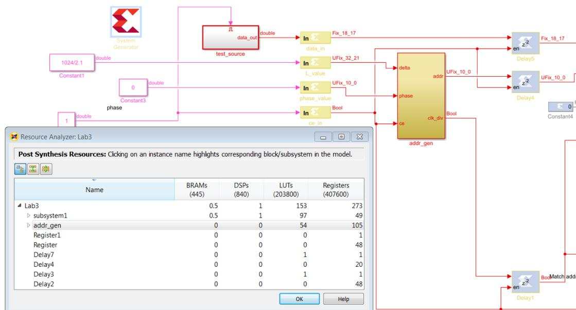
6. If the block or subsystem you have selected in the window is within an upper-level subsystem, then the parent subsystem is highlighted in red in addition to the underlying block as shown in the following figure.
