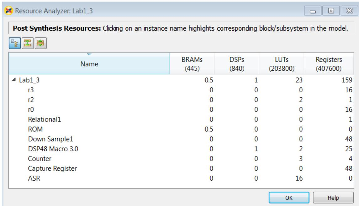
**Post Synthesis Resources:** Clicking on an instance name highlights corresponding block/subsystem in the model.
