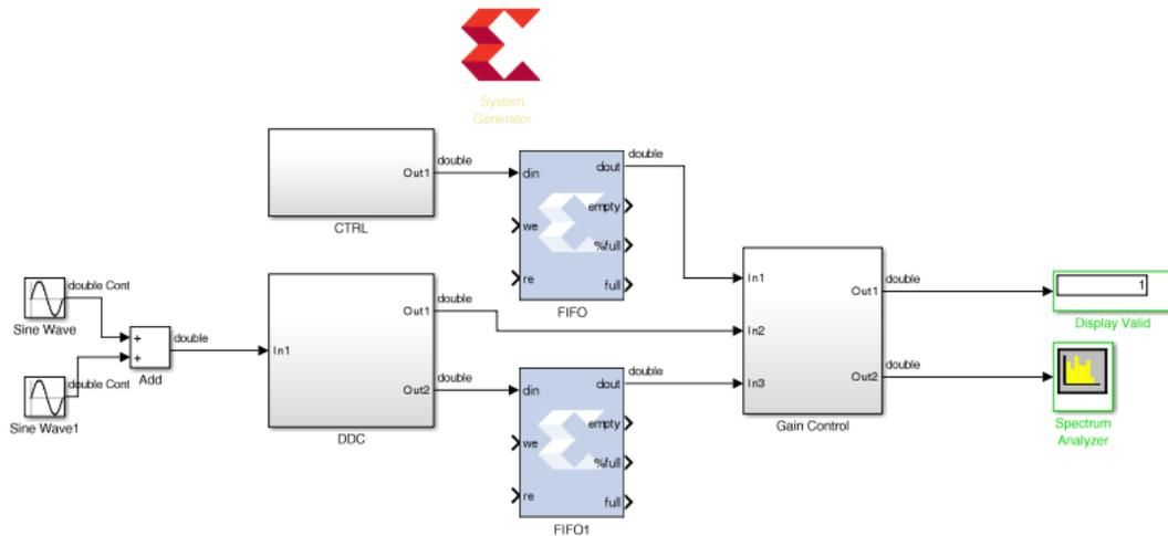
You will now connect up the control logic signals to ensure the data is safely passed between domains.
