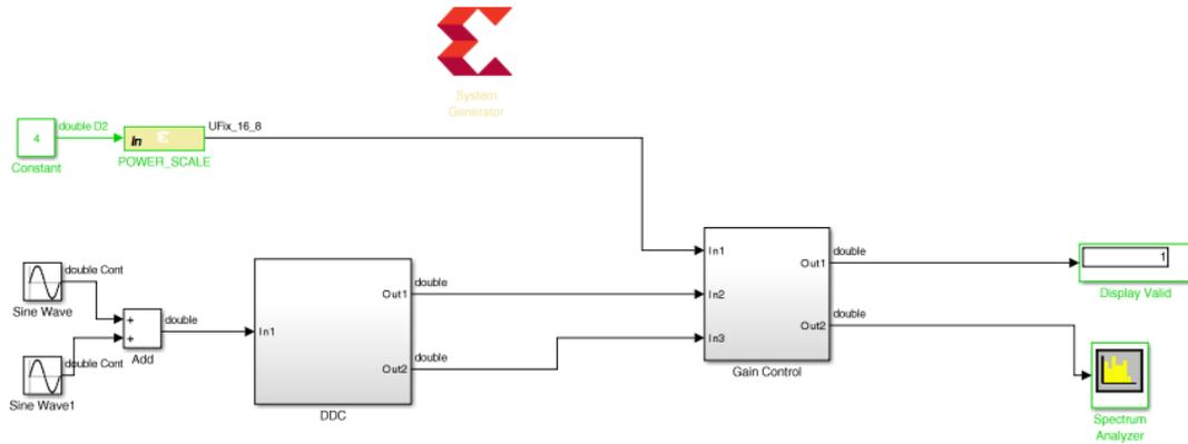
12. Finally, select the Gateway In instance **POWER\_SCALE** and **Constant** to create a new subsystem called CTRL. The final grouped design is shown in the following figure.
