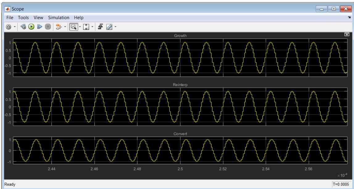
The Reinterpret and Convert blocks have not been configured at this point and so all three signals are identical.
