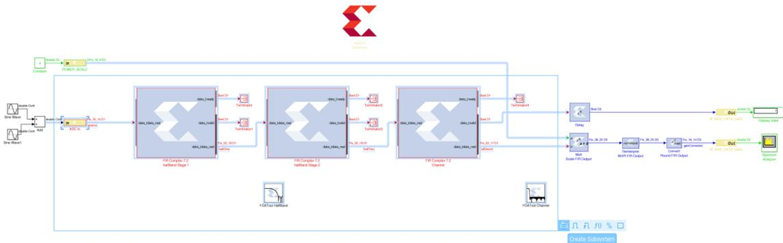
10. Select the instance name subsystem and change this to DDC to obtain the design shown.
