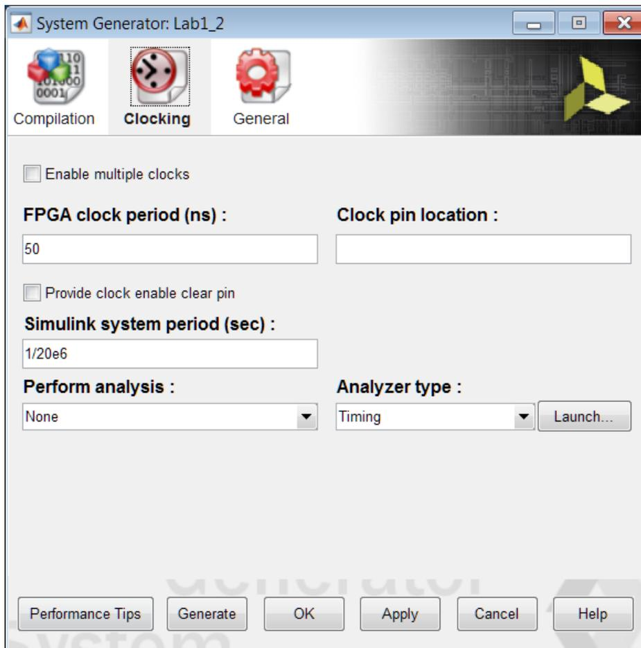
The frequency at which an FPGA device can be clocked easily exceeds 20 MHz. Running the FPGA at a much higher clock frequency will allow System Generator to use the same hardware resources to compute multiple intermediate results.
