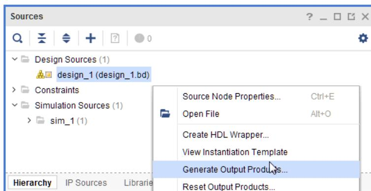
4. In the Generate Output Products dialog box, click **Generate** to start the process of generating the necessary source files.
