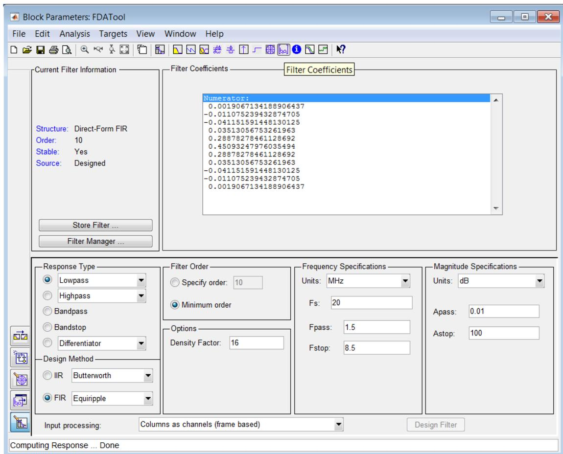
This shows the filter uses 11 symmetrical coefficients. This will require a minimum of six multiplications. This is indeed what is shown at the end of the Configure the System Generator Blocks section where the final hardware is using six DSP48 components, the FPGA resource used to perform a multiplication.
