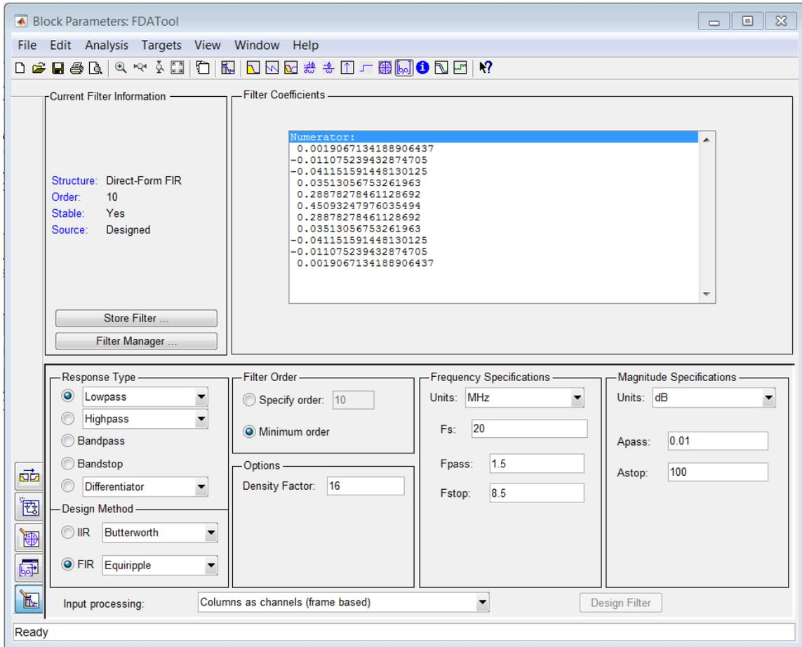
This shows the same specifications as the previous steps in Lab 1 and confirms there are 11 coefficients. You can also confirm, by double-clicking on the input Gateway In that the input sample rate is once again 20 MHz (Sample period =  $1/20e6$ ). With this information, you can now configure the discrete components.
