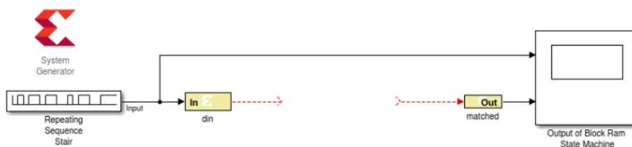
3. Add an MCode block from the Xilinx® Blockset/Index library. Before wiring up the block, you need to edit the MATLAB® function to create the correct ports and function name.
